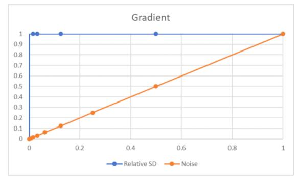
To test the equations, I have made several test images as well as using some actual astrophotos. The first is a smooth gradient which represents pure signal with no noise. The calculated SNR = 6440280.
