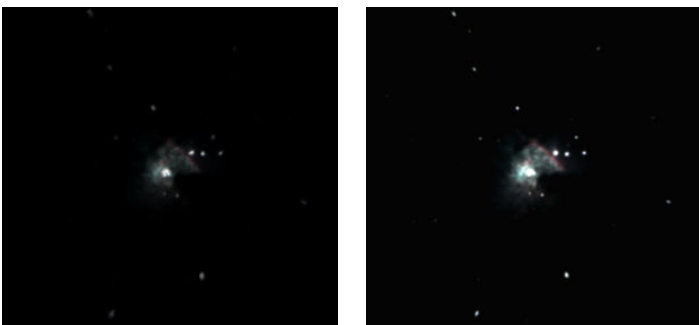
Example of the effects of a poorly collimated scope and a properly collimated scope - still using P&S digital camera.
