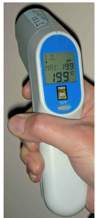
Right - infrared thermometer used for sky temperature readings
