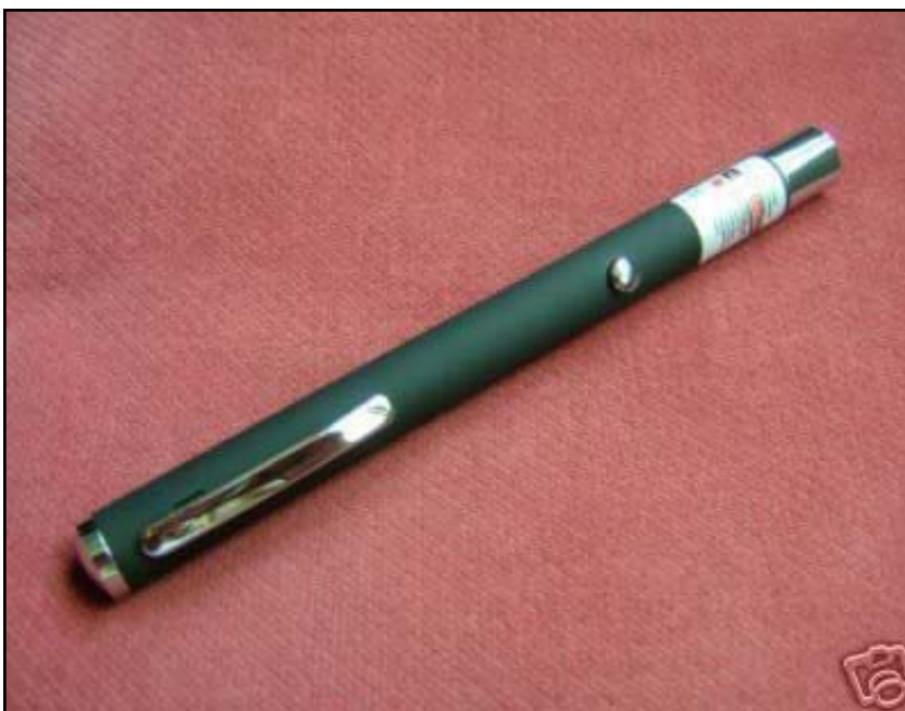
This is a typical LASER pointer used for astronomy. It has a 5mW output at 532nm which gives a brilliant green light. Easily portable in your pocket and uses two common AA batteries. Caution should always be used with these devices as they can easily cause eye damage if carelessly used.
