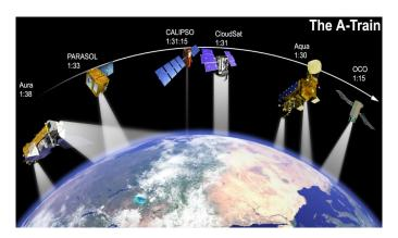
CloudSat, to be launched in November 2004, will take its place as part of the "A-Train" of satellites flying in formation to take closely timed snapshots of essentially the same scene using a total of 14 different measuring instruments.
