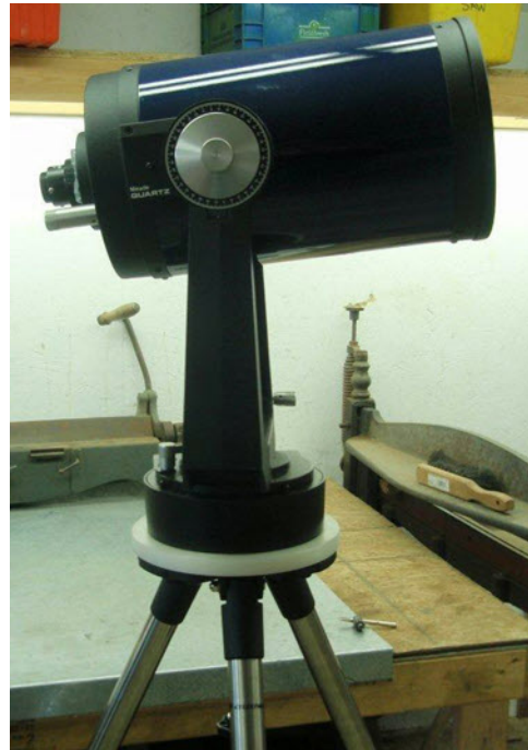
Left: Completed adapter with hole patterns to fit Meade telescope and Celestron tripod (shown below). Photos by the author.
