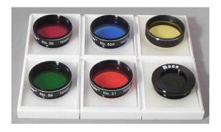
A set of planetary filters (R G B Y) and a good moon filter will greatly enhance your observing acuity. The planets have an intense brightness that filters selectively dim to enhance particular features: cloud bands, polar caps, etc..
