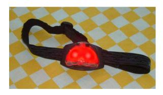
This hands-free flashlight has one red and two white LEDs (the red preserves your night vision). A switch turns on red or white light. I taped red plastic on my lights to make the white LEDs red as well. Several HAA members use these headbands while observing so they can illuminate their equipment while setting up with both hands.
